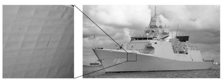
Additional costs for rework caused by weld-induced distortion: \$3Mio/ship
